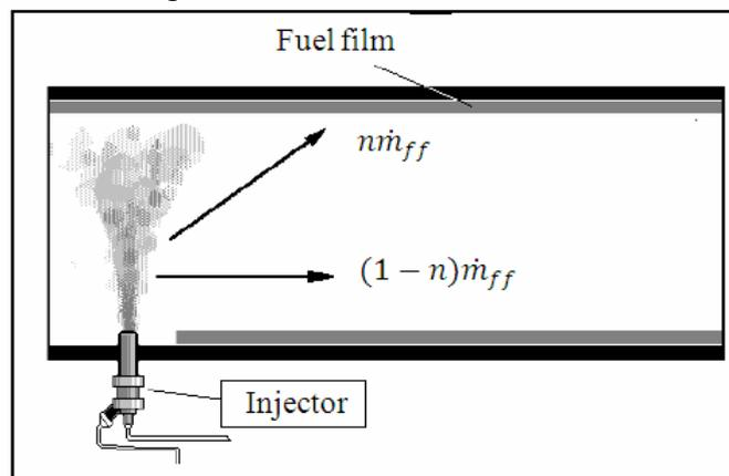
Figure 1 - Fuel film process in the intake manifold
